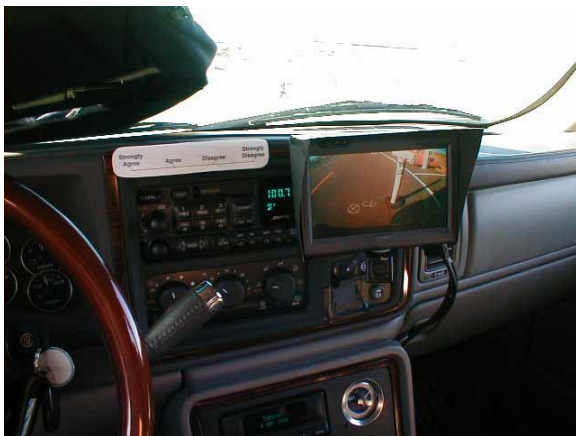
Figure 6. Parking aid experimental rear video display system.
