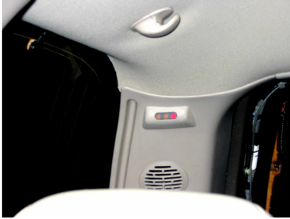
Figure 5. Passenger side rearmost pillar URPA visual interface.
