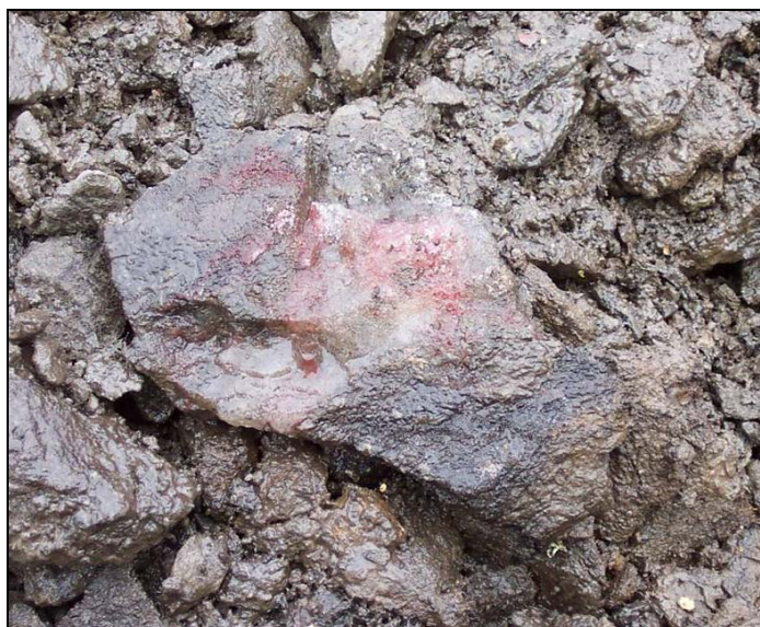
Figure 41. When alpha, alpha-dipyridyl dye is applied to a soil containing reduced iron, a positive reaction is indicated by a pink or red coloration to the treated area.
