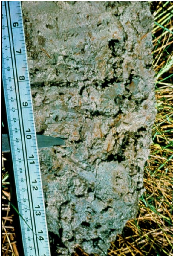
Figure 14. Indicator F3, Depleted Matrix. Redox concentrations are present within a low-chroma matrix.
