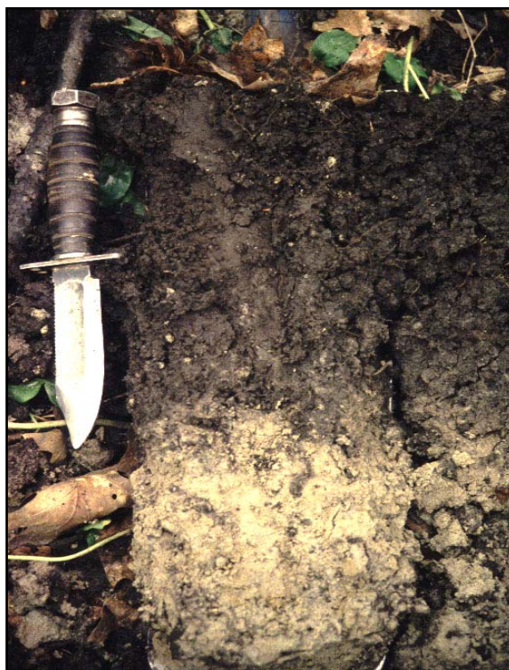
Figure 6. Depleted matrix starts immediately below the black surface layer (approximately 10 in. (25 cm)).
