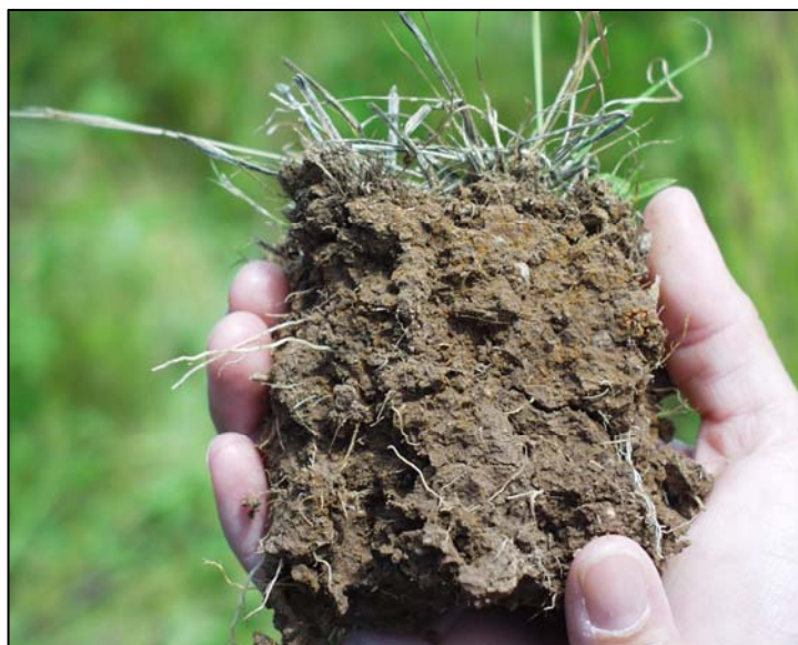
Figure 18. In this example, the layer of redox concentrations begins at the soil surface and is slightly more than 2 in. (5 cm) thick.
