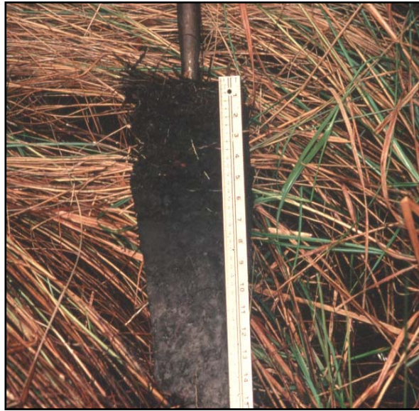
Figure 8. The mucky modified sandy layer is approximately 3 in. (7.5 cm) thick. Scale in inches on the right side of ruler.
