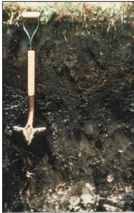
Figure 7. Deep observations may be necessary to identify the depleted or gleyed matrix below the dark surface layer.
