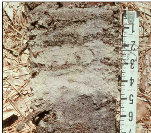
Figure 7. Stratified layers in sandy material. Scale in inches.
