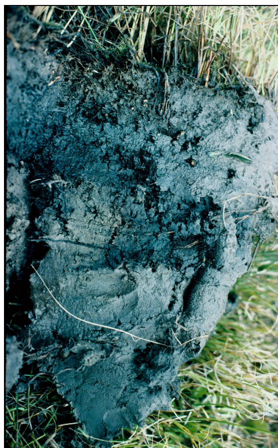
Figure 14. This gleyed matrix begins at the soil surface.
