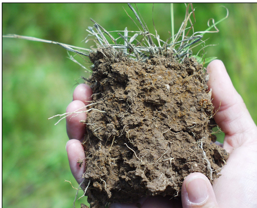
Figure 19. In this example, the layer of redox concentrations begins at the soil surface and is slightly more than 2 in. (5 cm) thick.
