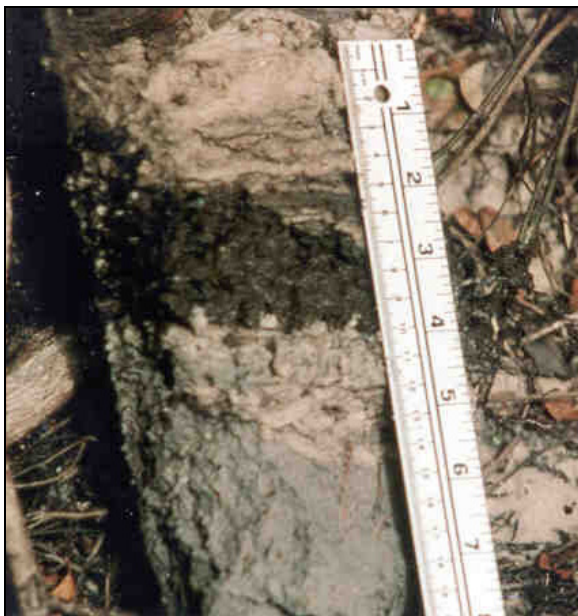
Figure 6. Stratified layers in loamy material.
