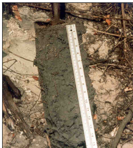
Figure 11. In this example, the gleyed matrix begins at the soil surface.
