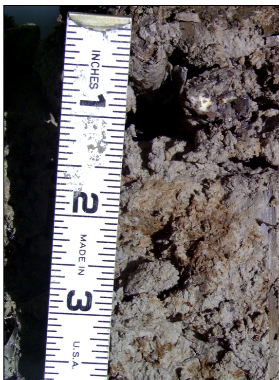
Figure 16. Redox concentrations at 2 in. (5 cm).
