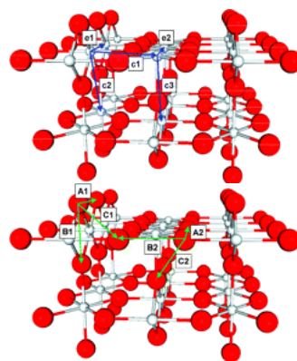
Figure 2. Electron (top) and hole (bottom) polaron transfer directions at the rutile (110) surface.
