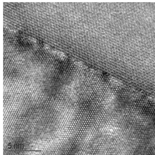
Figure 1. High-resolution transmission electron microscopy image showing the interface between \alpha - \text{Al}_2\text{O}_3 and ZnO with the film grown on r-cut \alpha - \text{Al}_2\text{O}_3 .
