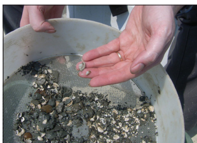
Photo, bottom right: Sediment samples were screened for paint chips and other debris. Some samples contained large amounts of juvenile resident clams.
