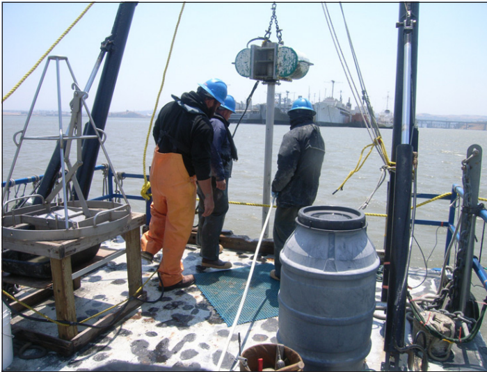
Photo, above: Scientist deploying Vibracore for sampling.
