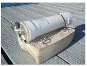
Figure 8. The EAR attached to a concrete anchor
