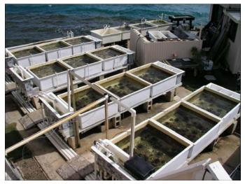
**Figure 16.** Ocean acidification experiments being conducted in mesocosm facility at Coconut Island. Projected future levels of acidification were produced by pumping dilute acid into the intake.
