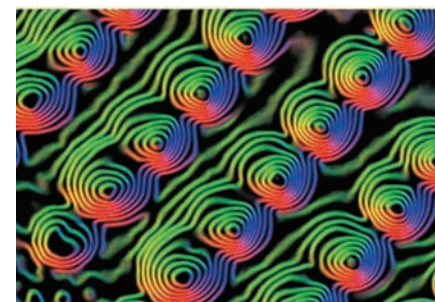
Electron microscopes create greatly magnified images by recording how a beam of electrons interacts with a sample material. Above is such an image, showing nanostructured magnetic nickel. Such materials could someday be used in data storage, electronics, biomedicine and telecommunications.
