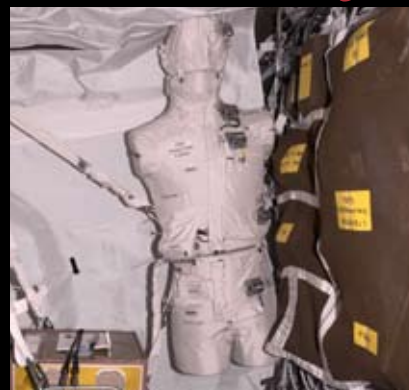
Bonner Ball Neutron Particle Detector and Phantom Torso for radiation measurement experiments.
