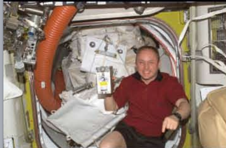
Crewmember Mike Fincke holds an RPCM in the Quest Airlock. It was later used to replace an RPCM on the S0 Truss.
