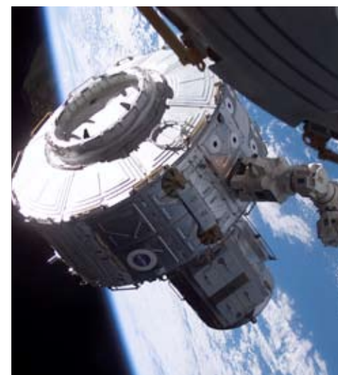
Space Shuttle mission STS-104 berths Quest to the starboard side of Node 1 in July 2001.
