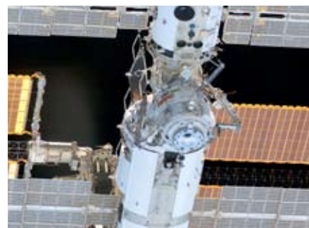
Pirs Module location at Service Module nadir.
