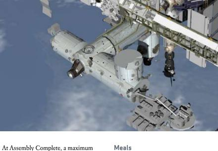
At Assembly Complete, a maximum 110 kW of power, including 30 kW of long-term average power for applications, is/will be available.
