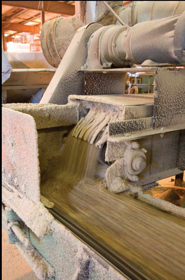
Pellet mill open for business @ 4 tons per hour
