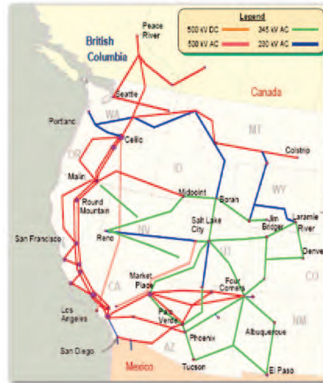
Figure 2-3: Primary Components of the WECC Transmission Grid
