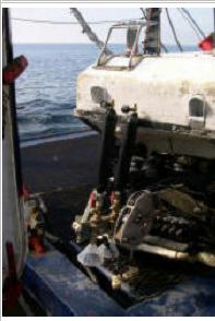
Samples are also recovered using the ROV's (remotely operated vehicle) mechanical arm and are brought to the surface for analysis.
