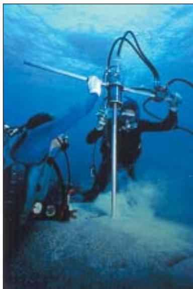
Researchers use a hydraulic drill to collect a core from coral. Corals often live hundreds of years and are useful in documenting climatic change.
