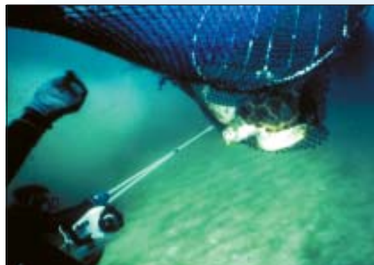
Fishing gear experts evaluate the effectiveness of a turtle excluder device (TED) in action.
