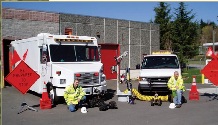
Closed circuit television equipment is used to check conditions of some wastewater pipes.
