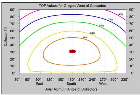
Draw a dark **X** mark the graph for your collector's tilt and azimuth angle. Interpolate between the nearest two lines to estimate the TOF value to the nearest 1%.
