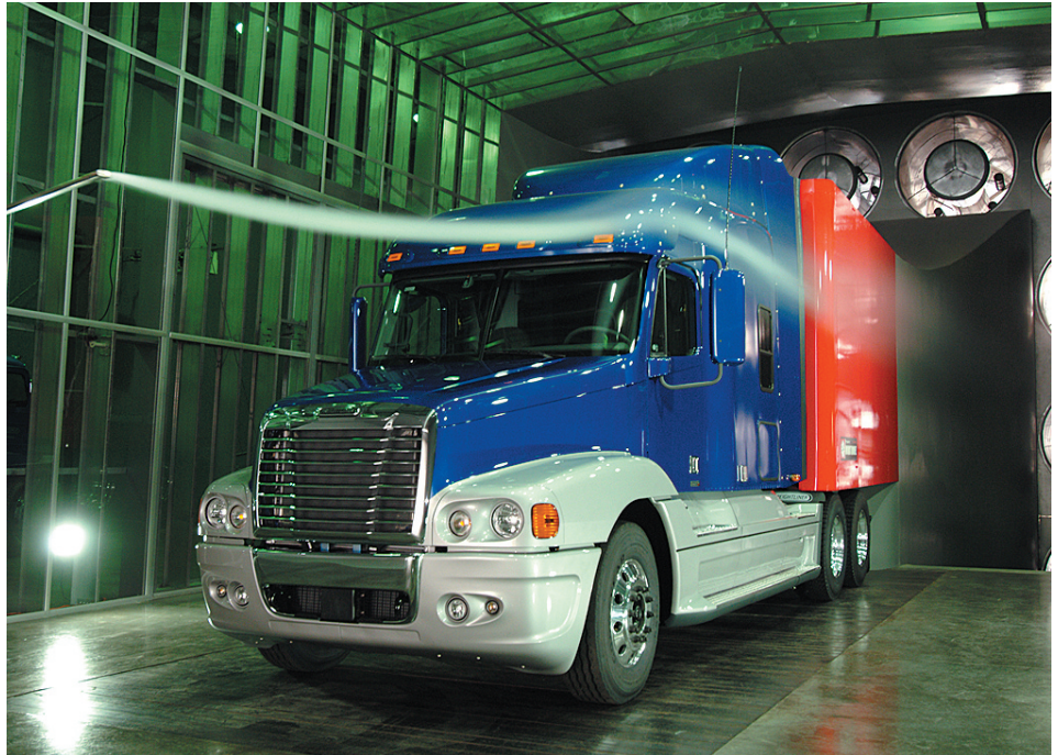
Testing shows airflow direction over a Freightliner truck in the new Freightliner Wind Tunnel Research Facility. Photo courtesy of the Oregon Department of Energy.
