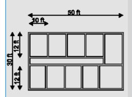
W. Using the tenant space method, the interior lighting power allowance is 1,500 sq. ft. x 1.0 W/sq. ft. = 1,500 W. Using the space-by-space method, the allowance for the enclosed offices is 1,350 sq. ft. x 1.1.W/sq.ft. = 1,485 W. The allowance for the corridors is 150 sq. ft. x 0.5 W/sq. ft. = 75 W. The total allowed interior lighting power is 1,560 W.
