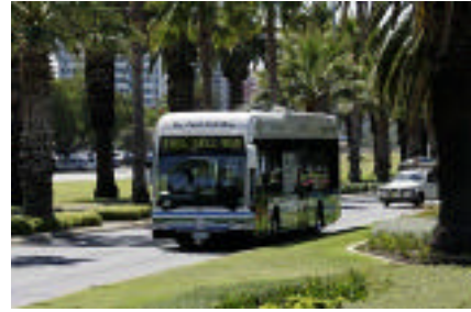
40-Foot DaimlerChrysler EvoBus with Ballard Fuel Cell in Perth, Western Australia
