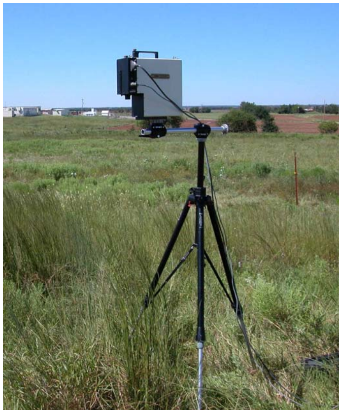
Figure 1. GER3700 setup used for surface reflectance measurements during the IOP.
