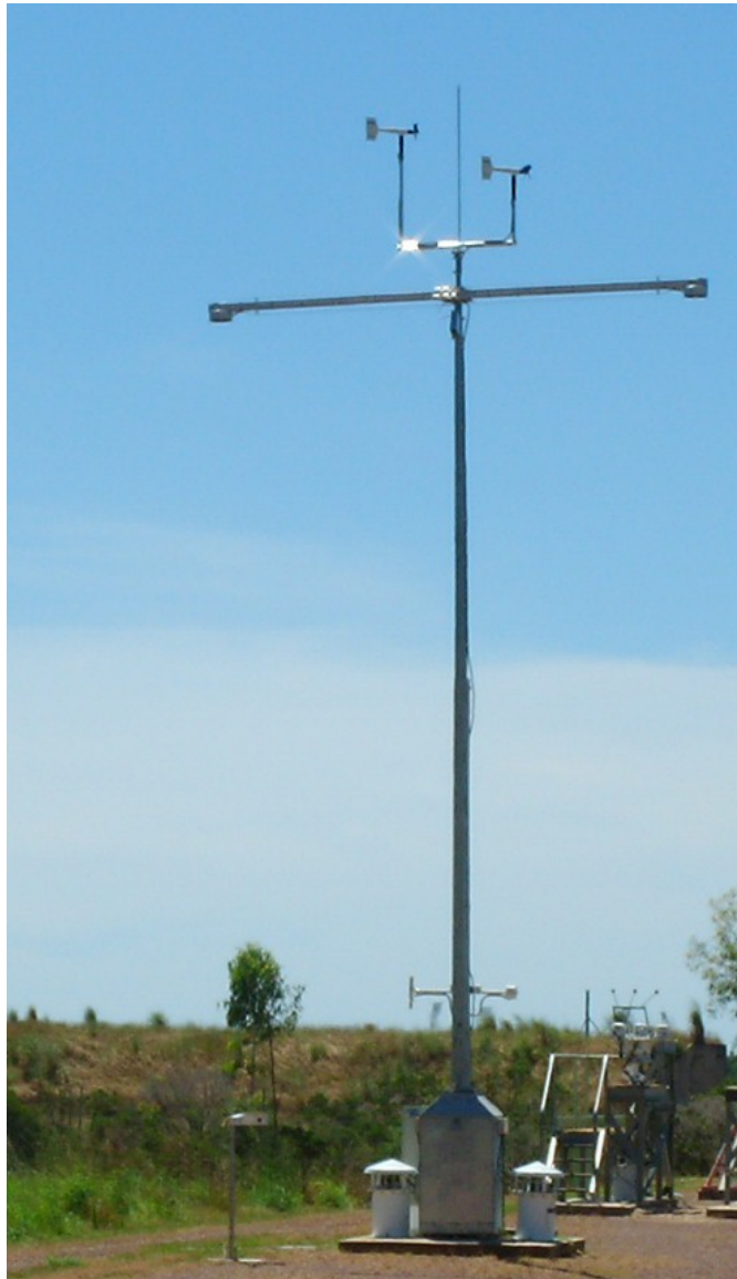
Figure 2. Surface meteorology system at the TWP site in Darwin, NT, Australia.
