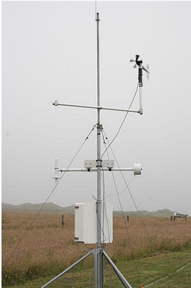
Figure 5. ARM Mobile Facility Surface Meteorology station set-up.
