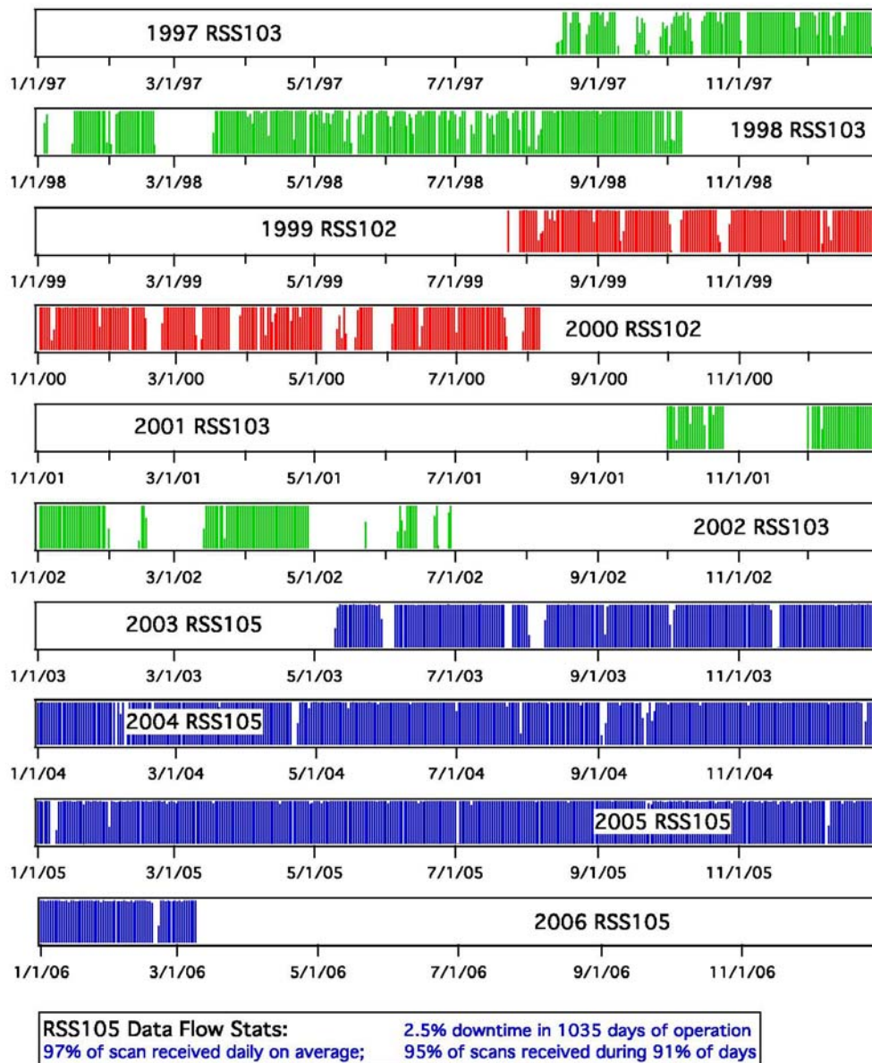
Figure 3. Data availability from two RSS prototypes (RSS102 and RSS103) and from the presently deployed RSS105.
