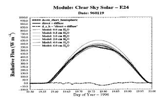
**Figure 1**. Display of SIROS derived estimates of the hemispheric broadband and modeled estimates for the Cyril, OK Extended Facility on January 19, 1996. 40 W m<sup>-2</sup> differences between the unshaded pyranometer (down\_short\_hemispheric) and that calculated from the direct and diffuse components are noted during mid-day.
