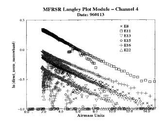
**Figure 3.** MFRSR Channel 4 natural logarithm (direct radiation) plotted as a function of airmass reveals the expected linearity for a given EF as a function of nearly clear sky conditions across the SGP Site. Values near -1 for the irradiance indicate "missing" data points.
