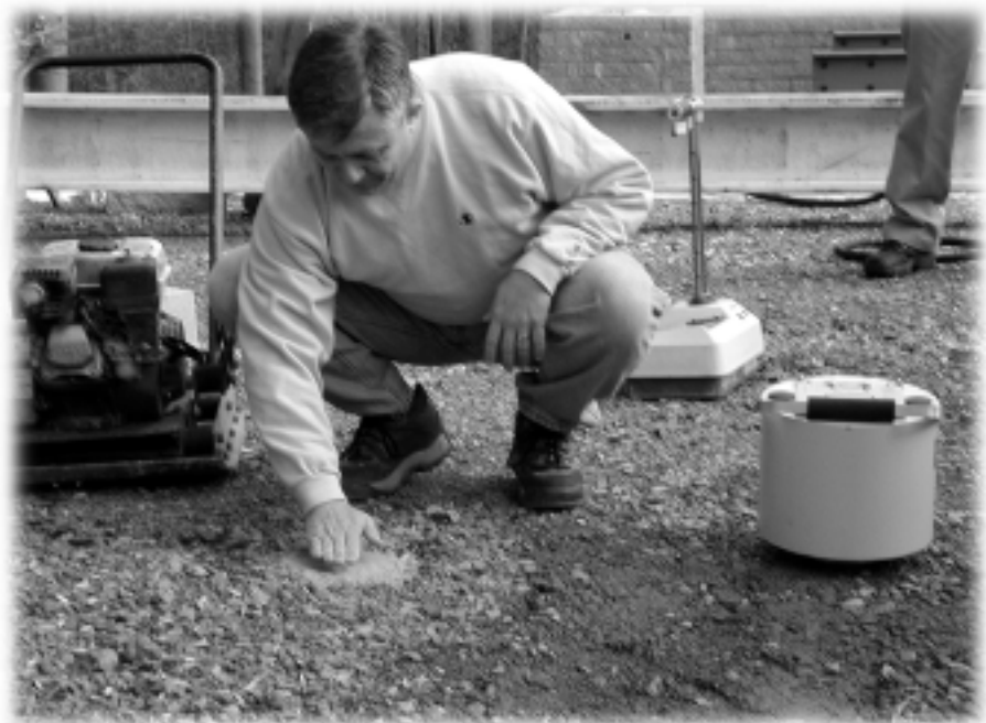
Melvin Main, who helped develop the device on the right known as the SSG, prepares the ground with a thin layer of sand to perform a soil stiffness test.
