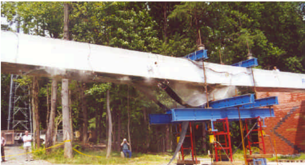
The fiber-composite plates debonded at the conclusion of the test. This photograph was taken at the moment of failure.
