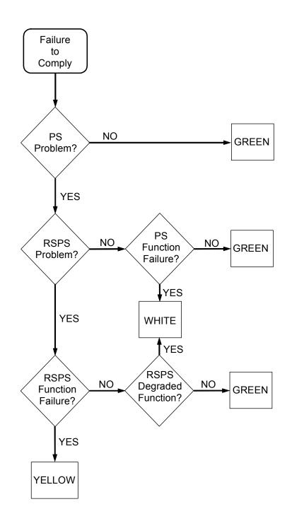
NOTE: PS/RSPS Function Failure is equivalent to LOSS OF PS/RSPS FUNCTION
