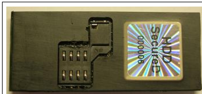
Figure 3 SecureD FPGA Sample (front) - Epoxy Coated with Tamper Sticker Sample
