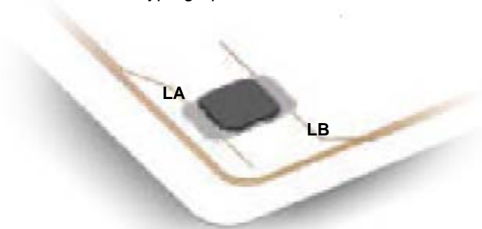
Figure 5: Example of connection of the cryptographic module to the antenna for the contactless mode
