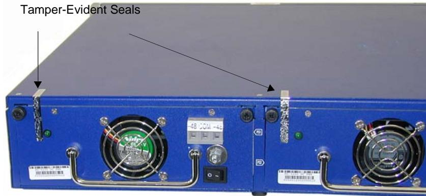
**Figure 2** Tamper Evident Mechanisms
