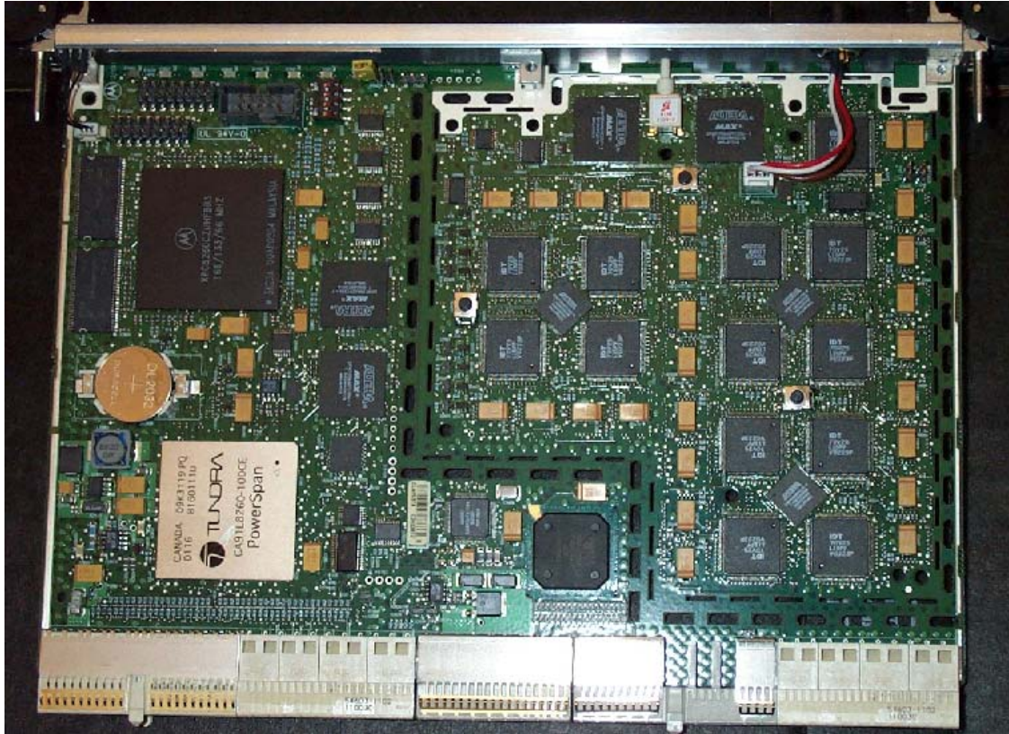
Figure 1: MGE SC front w/o tamper shield. Crypto boundary defined by dashed 'line'.
