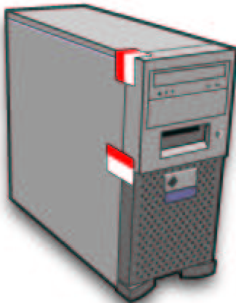
Figure 3.1: Tamper-evident Label Placement on a Sun SPARC Ultra-10.
