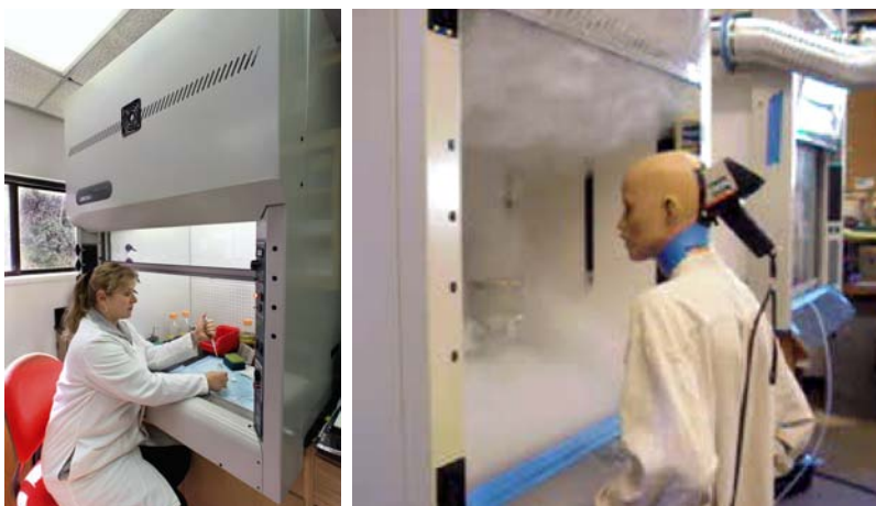
Figure 8. Prototype high-performance fume hood. Air is introduced in the frame (“face”) of the hood, in front of the worker (see grill under right wrist), maintaining or improving containment and reducing energy use. Typical designs draw air from the general lab space around the worker, causing turbulence and higher-than-necessary fan energy use. Smoke in right panel shows air entering through the frame.
