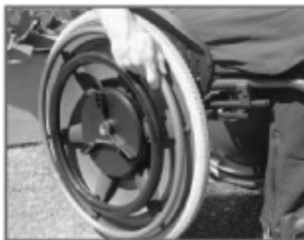
Magic Wheels' new 2-speed geared manual wheelchair wheel. See www.magicwheels.net for details.
