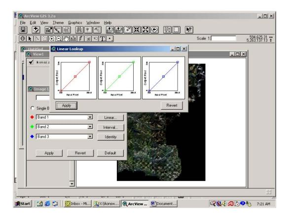
The 'Linear Lookup' dialog displays a color lookup graph for each of the Red, Green and Blue display bands for the imagery. Although you are free to experiment with adjusting the bands independently of one another, adjusting each lookup approximately the same amount will provide the most consistent results.
