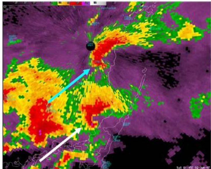
Fig. 9. KAMX 0.5-degree base reflectivity image at 0145 UTC 2 Jun 2007; Card Sound (Cutler Ridge) mesocyclone denoted by white (blue) arrow.
