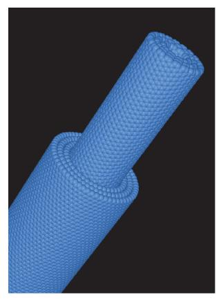
Model of a multiwall carbon nanotube whose inner set of tubes has been "telescoped" out. This sliding motion is theoretically predicted and experimentally demonstrated to be almost frictionless. The tubes thus could constitute an ideal nanoscale bearing or constant force spring.
