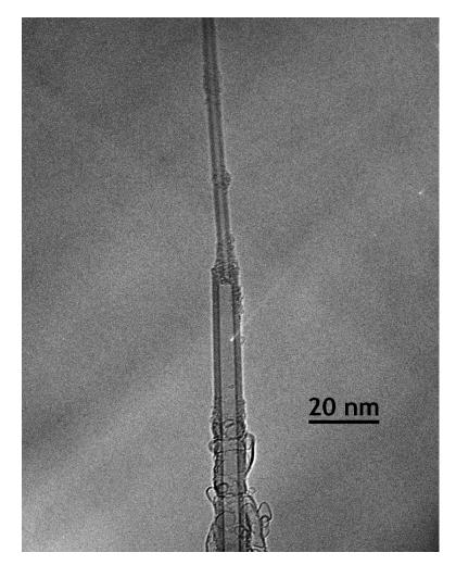
Transmission electron microscope image taken at the LBNL National Center for Electron Microscopy of a "telescoped" multiwall carbon nanotube. No atomic-scale degradation is observed with repeated extensions and retractions. The system may thus be wear-free with no fatigue.
