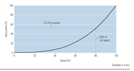
A VSD is not a motor; it is an electronic device that varies the speed of a motor by changing the frequency of the electrical power between 0 and 60 Hertz. The EPA study "Variable Air Volume Systems Maximize Energy Efficiency and Profits" showed that VSDs can greatly reduce the energy used by the same fan operating under similar airflow volumes and static pressure conditions. Overall, the study indicated that VSDs provided an average energy savings of 52 percent.
