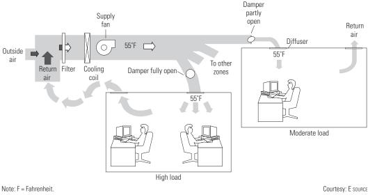
A proper conversion to a VAV system includes changing constant-volume dampers to operate in variable-volume fashion, which typically reduces fan horsepower requirements by 40 to 60 percent. Conversion from constant to variable volume can be complicated in certain circumstances due to nonmechanical factors such as:
