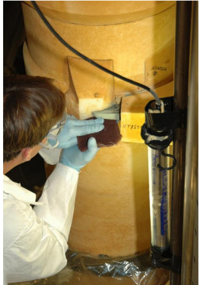
The super lightweight ablator, or SLA, cork insulation has been removed from the external tank and a United Space Alliance external tank technician sands off the residue from the LO 2 feed line bracket. The BX265 foam insulation was later reapplied without the SLA.
