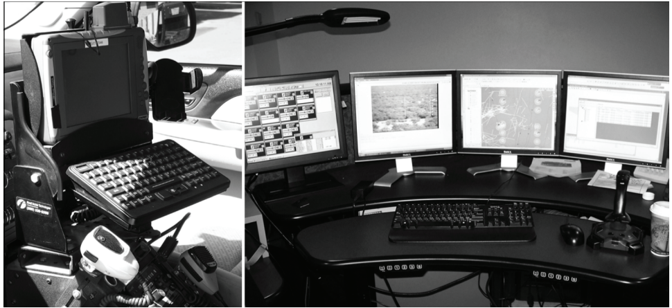
Figure 3: At Left, Mounted Laptop Installed in Border Patrol Vehicle; at Right, Project 28 Command and Control Center
