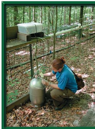
Integrated air samples taken every 2 weeks are used to interpret isotopic signals of carbon flux.
