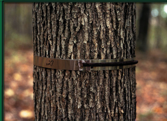
A dendrometer band is used to make short-term, repeated measurements of changes in diameter of trees.
