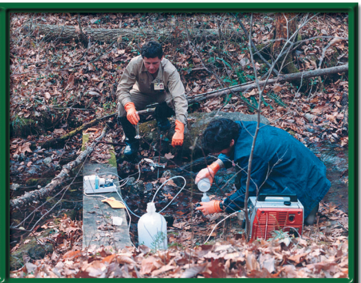
ORNL researchers inject a radiotracer as phosphate into Walker Branch to study the uptake and cycling of phosphorus in streams.
