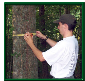
A student determines tree diameter as part of a project testing the ability of an experimental airborne radar to remotely measure tree biomass. (Photo by Liz Williams.)
