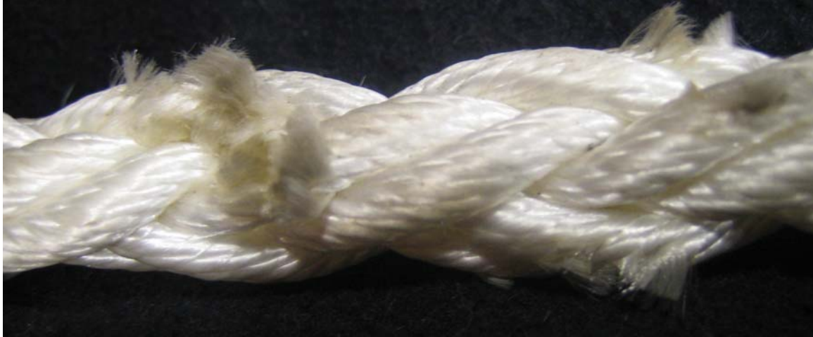
Figure 19: \frac{3}{4} " 8-strand plaited nylon: KEO recovered nylon cut fiber patch.
