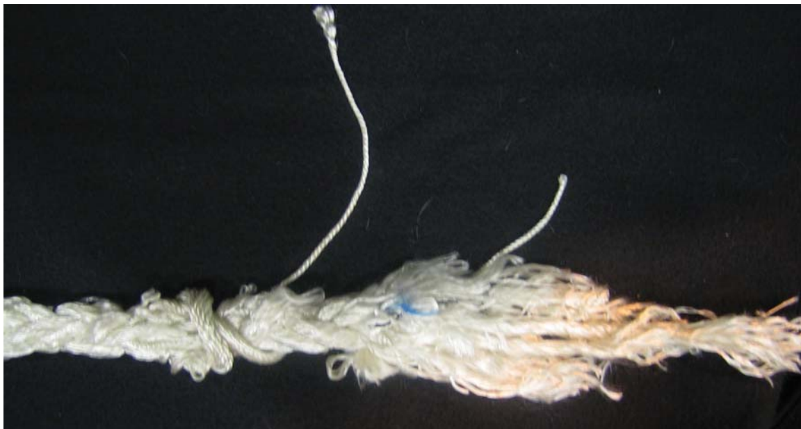
Figure 17: 3/4'' 8-strand plaited nylon: section F–G parted end.
