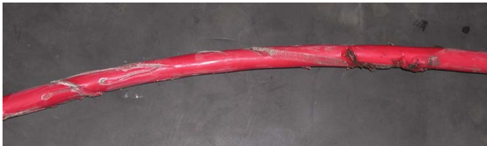
Figure 29: Damage to 3/8'' jacketed wire rope at a depth of \sim 547 m.
