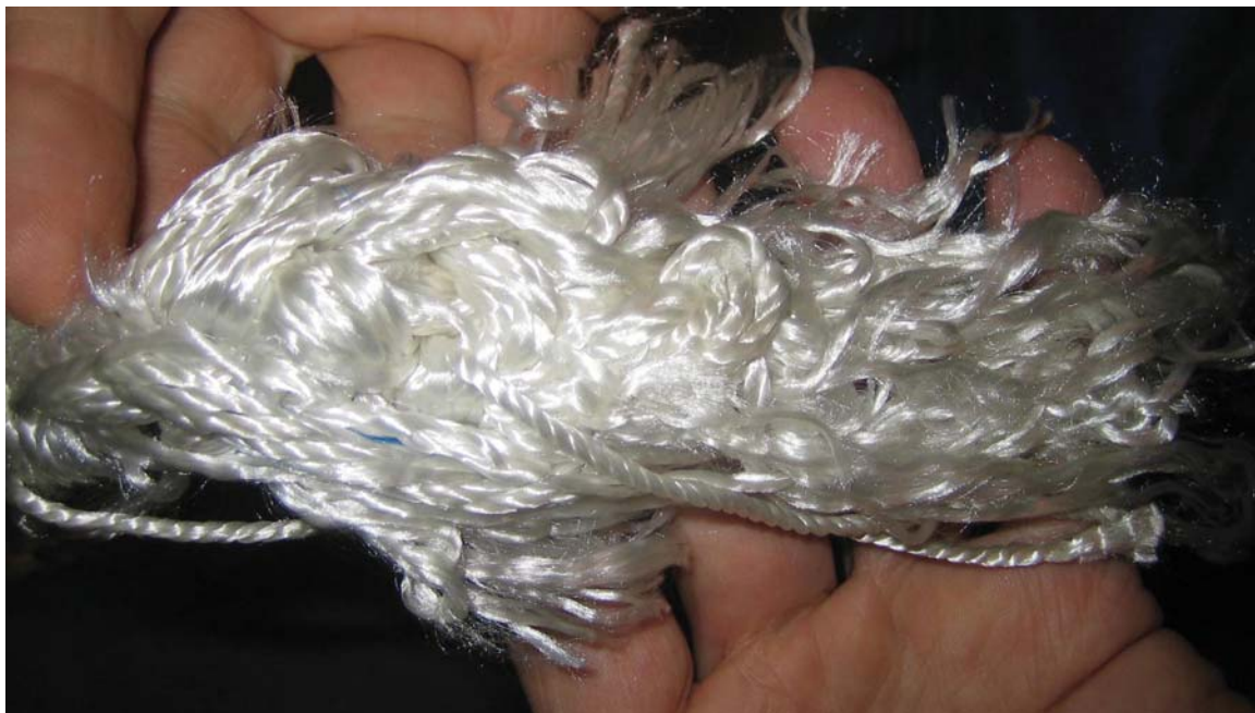
Figure 18: 3/4'' 8-strand plaited nylon: section G parted end.
