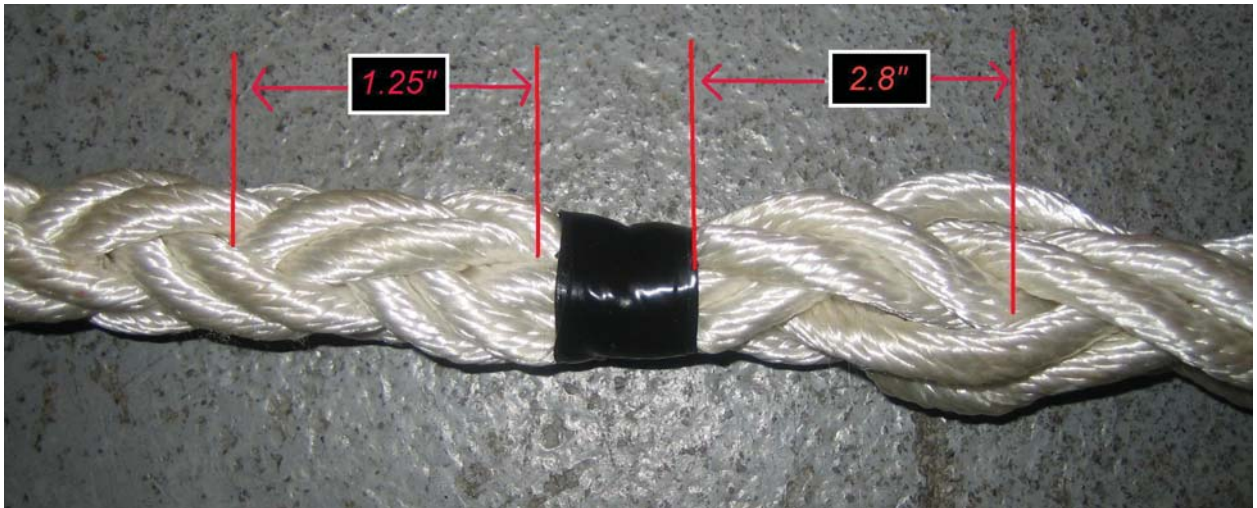
Figure 11: \frac{3}{4} " 8-strand plaited nylon: section A change in pik length.
