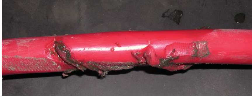
Figure 28: Damage to 3/8'' jacketed wire rope at a depth of \sim 547 m.
