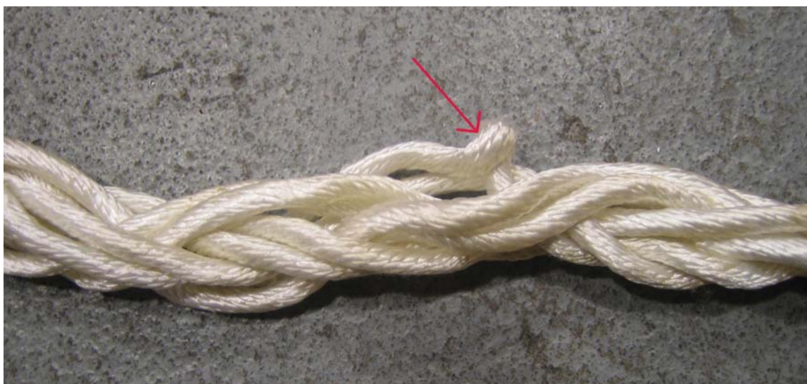
Figure 14: \frac{3}{4} " 8-strand plaited nylon: section C kink.
