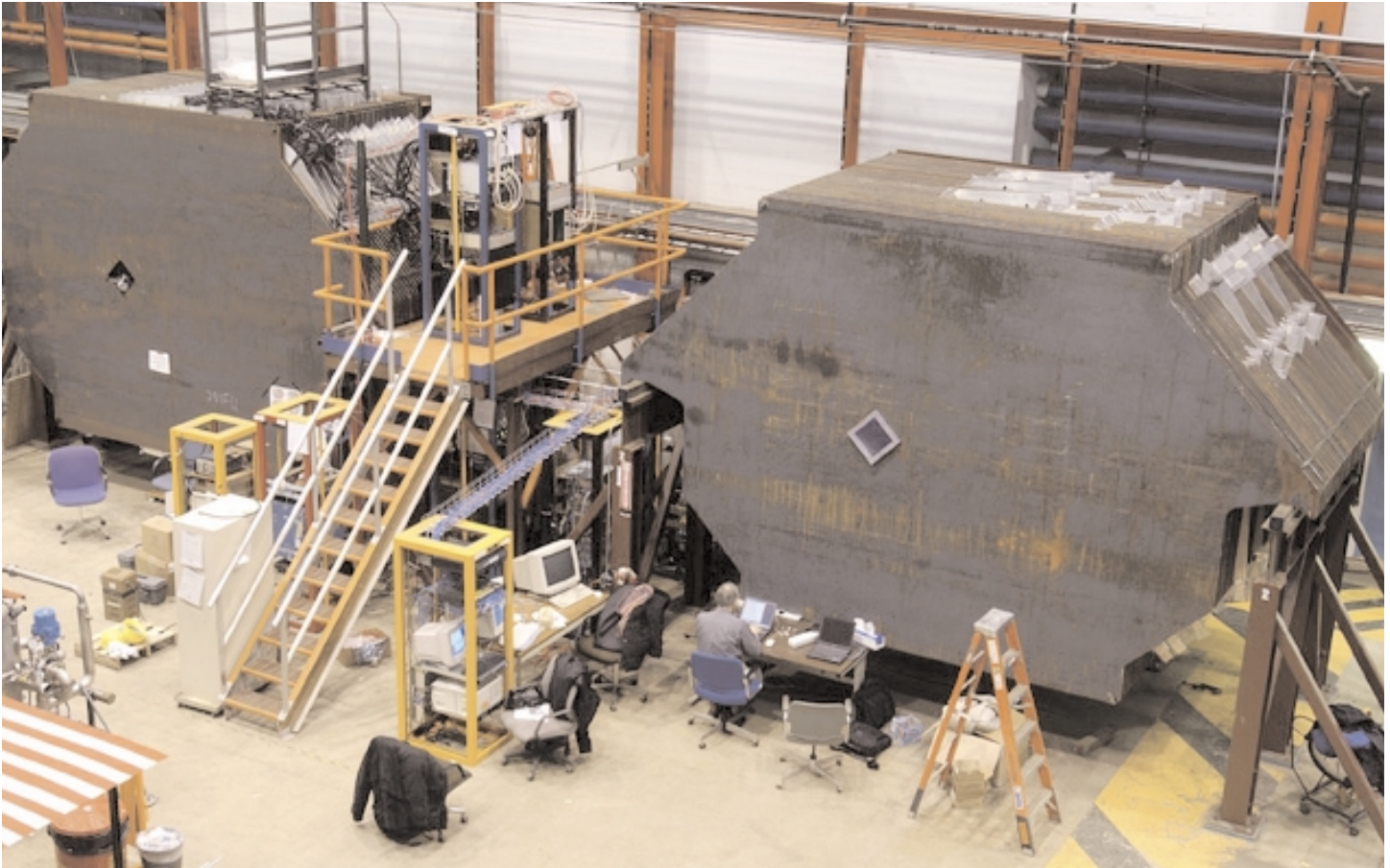
The 282 detector planes for the MINOS near detector are in storage in a large experimental hall at Fermilab. Scientists are currently practicing the setup of the data acquisition system on nine of the planes.
