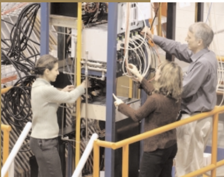
At the end of February the test stand of the MINOS data acquisition system at Fermilab recorded the first cosmic rays. Niki Saoulidou (left, Fermilab), Simona Murgia (Stanford University) and Geoffrey Pearce (Rutherford Laboratory) are some of the scientists who've worked on setting up the installation.
