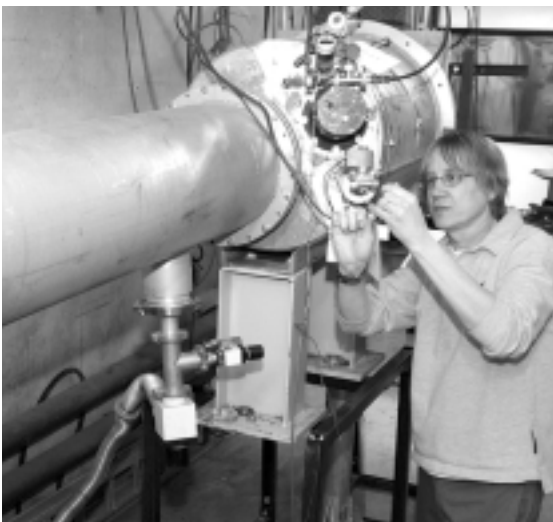
The beam line to the Meson Test Beam Facility can deliver a variety of particles. A particle identification system, built by Erik Ramberg, informs experimenters about the types of particles delivered to their test stands.
