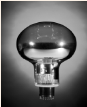
One of the 8-inch PMTs used in the MiniBooNE detector. The Super-K PMTs are much larger, 22 inches in diameter, and are hand-made by glassblowers and therefore very expensive to replace. A 22-inch PMT costs around $3,000.
