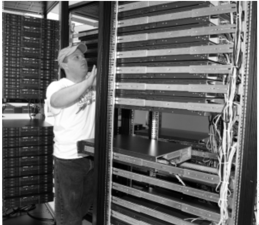
Atipa representatives installed the units in the racks at Feynman Computing Center. Computing administrators booted up the systems, one unit at a time, and began the 30-day “burn-in” with a suite of software tools designed to stress the various hardware components (CPU, memory, disk, network).
