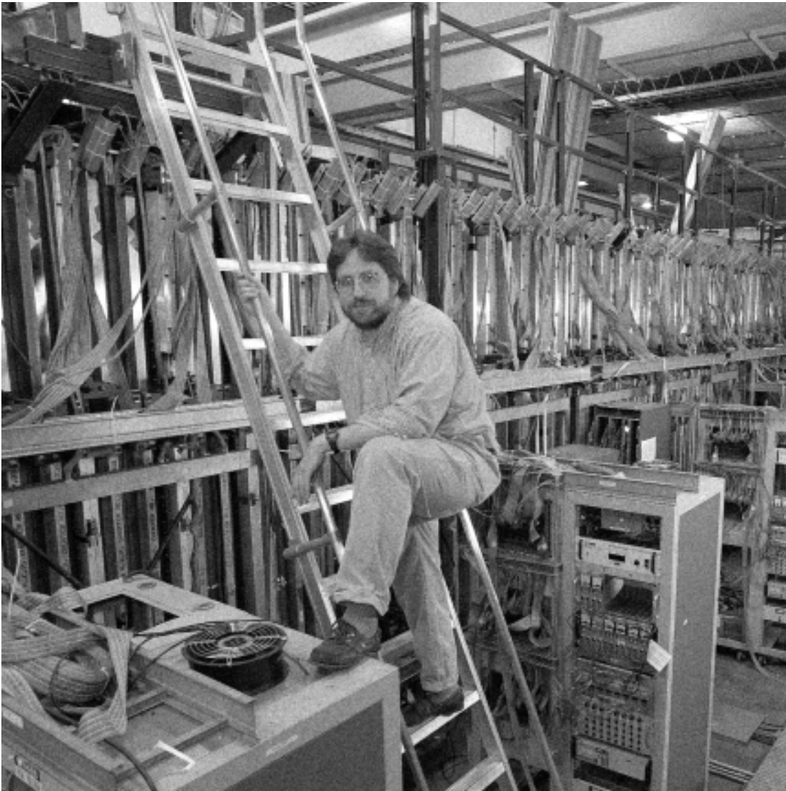
Fermilab physicist and NuTeV spokesperson Bob Bernstein with the NuTeV detector, a 700-ton sandwich of steel, scintillator and drift chambers.
