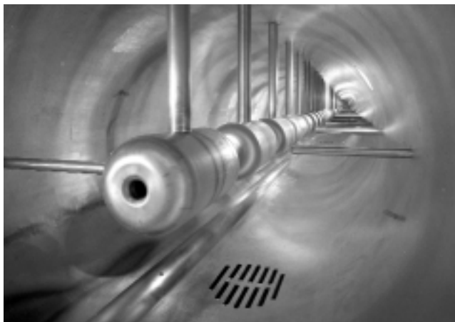
The interior of the linear accelerator at Fermilab. The copper structures get charged using alternating voltage to accelerate particles.
