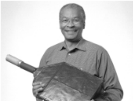
Herman White with a particle detector made of plastic scintillating material, which detects charged particles as they pass through a counter.
