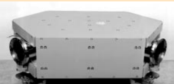
This magnet bends the electron beam 90° for injecting and extracting with almost no disturbance to the antiproton beam.
