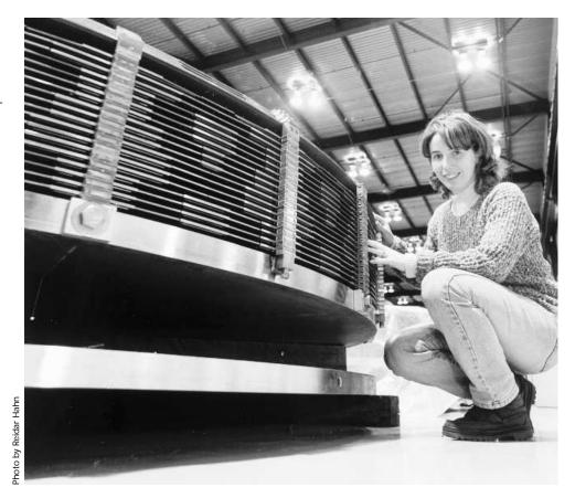
sors, along with their students and an engineer and research associate, are developing and testing the upgrade to the endplug and the calorimeter's optics system. This system, drawing upon technology similar to the fiber optics in phone lines, uses scintillation and optical fibers to capture light and reconstruct information about interesting particle interactions that occur in the detector.
